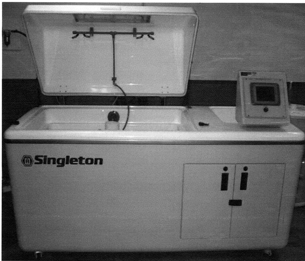
Photograph 3 Cyclic Corrosion Test Chamber
