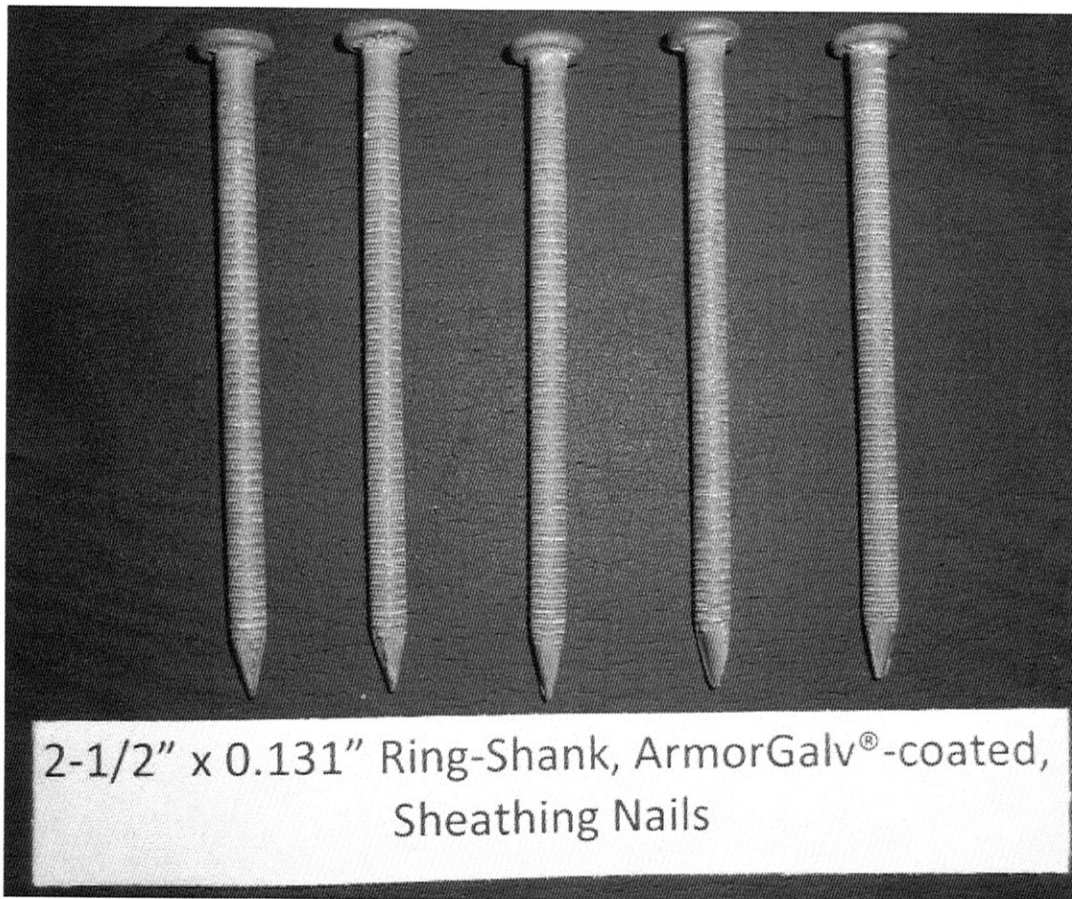
Photograph 6 2-1/2" x 0.131" Ring-Shank, ArmorGalv®-Coated, Sheathing Nails (After)
