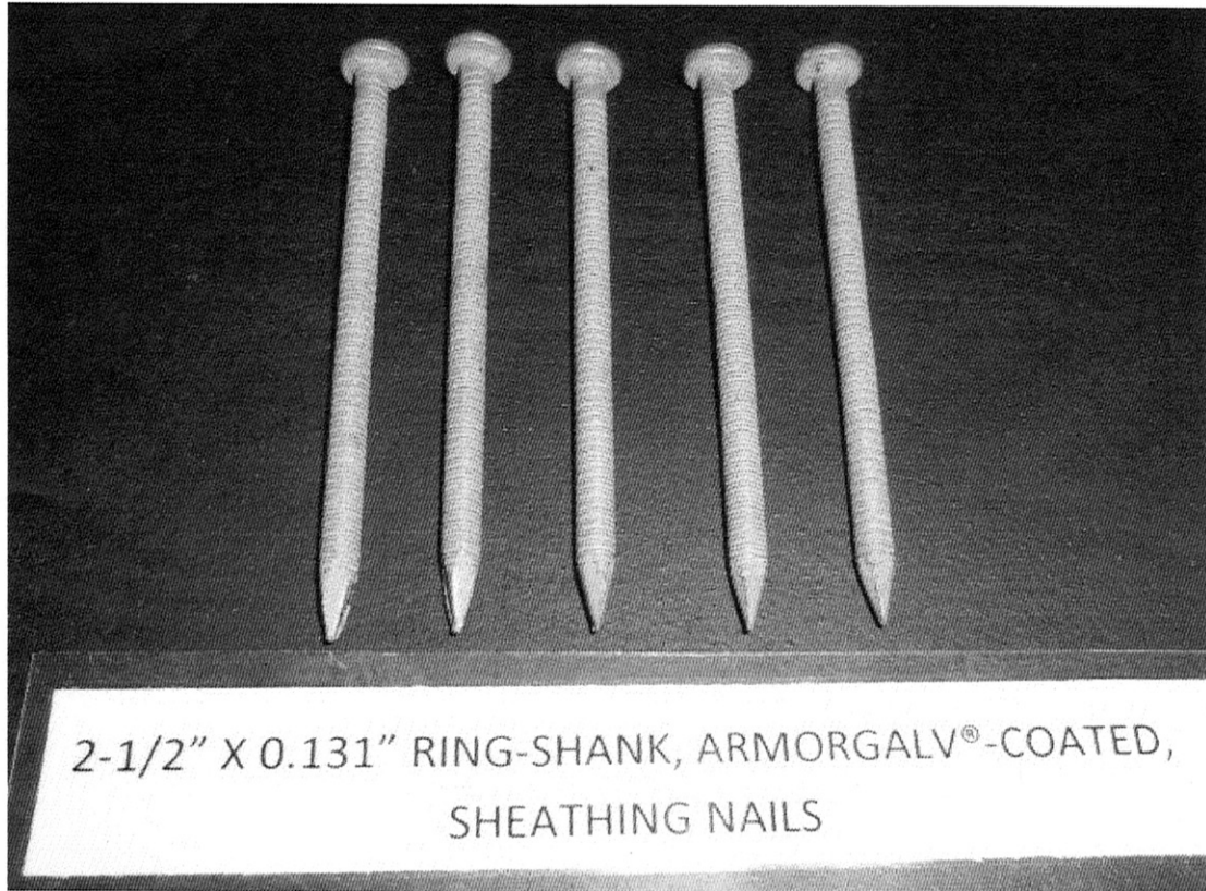
Photograph 2 2-1/2" x 0.131" Ring-Shank, Armorgalv®-Coated, Sheathing Nails (Before)
