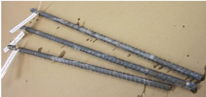
Figure 4 ArmorGalv® process after 3000 hours in salt fog exposure
