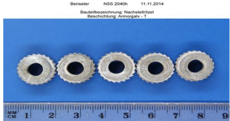
Sintered steel ratchet wheels (2040 Hrs salt spray)
