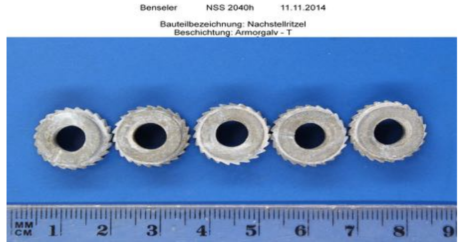
Sintered steel ratchet wheels (2040 Hrs salt spray)
